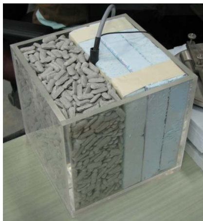
Figure 4. Measuring thermal conductivity of pellet fill using a one-sided test configuration.
