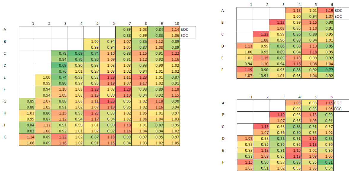
Figure 2 Normalized radial power distributions (1/4 core) for the beginning (BOC) and end of cycle (EOC) for the SCWR (left), SSR (top right) and short core SSR (bottom right).
