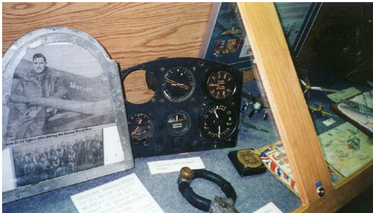
Figure 2 - Radium bearing gauges in museum display case
