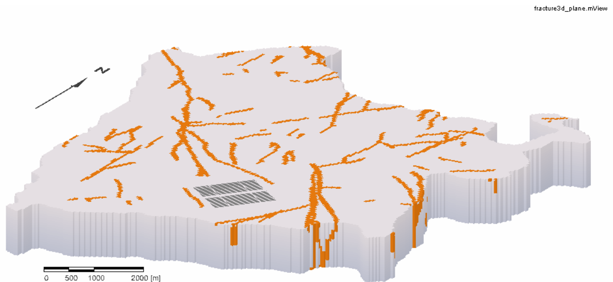
Figure 4: Cutaway view of rock mass under the watershed at the repository horizon of 660 m depth, showing the major fractures and repository location.
