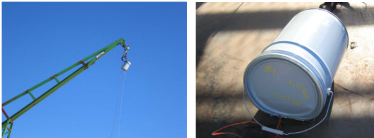
Figure 10. Drop Test of Metal Pail (Nalgene Bottle Inside) from 9 m.
