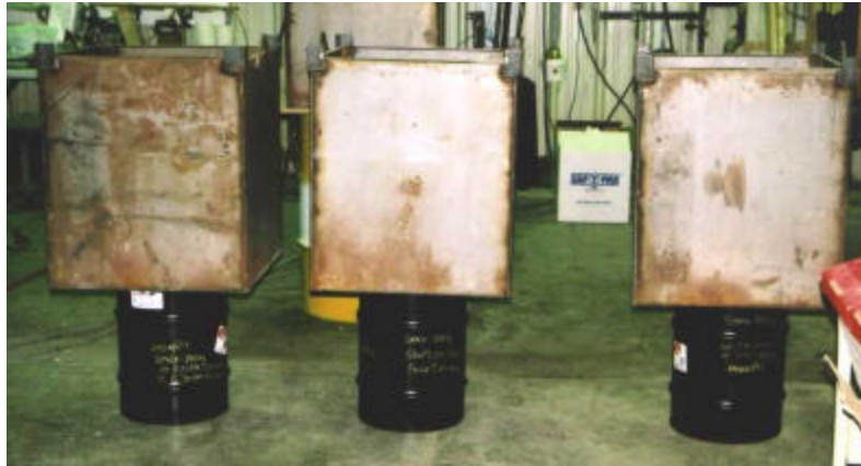
Figure 9. Stacking Test (10 Gallon Drums)
