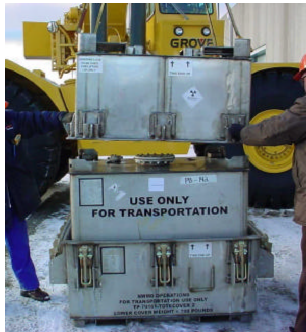
Figure 12. Stainless Steel Tote and Tote Overpack
