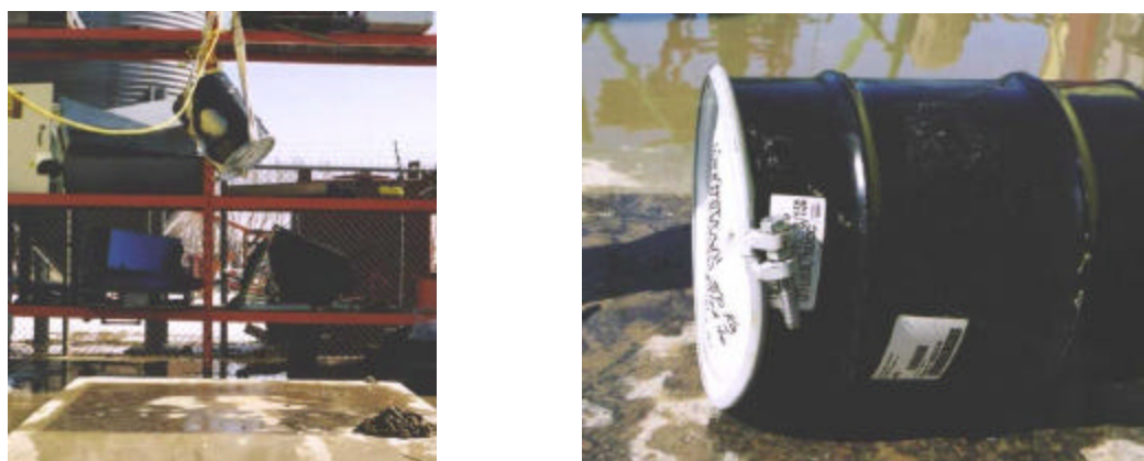
Figure 8. Corner Drop Test for the 10 Gallon Drum
