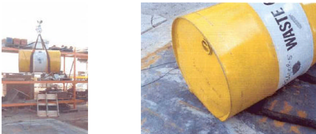
Figure 7. Side Drop Test for the 45 Gallon Carbon Steel Closed Head Drum (#1)
