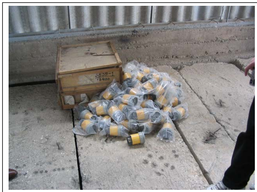
Figure 3: New batch of used smoke detectors, containing very small quantities of ^{239}\text{Pu}
