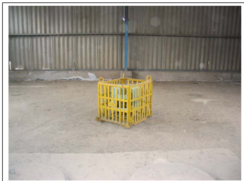
Figure 2: Radioisotope thermoelectric generator, originally containing 30 000 Ci of ^{90}\text{Sr}
