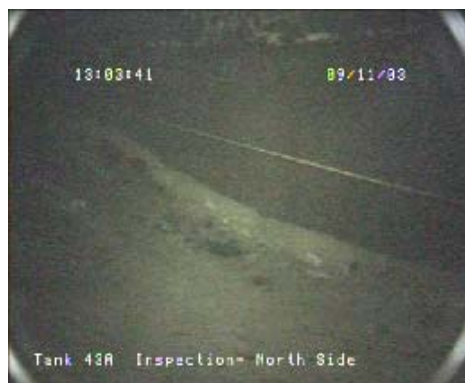
Figure 9: Variation in Depth of Sludge
