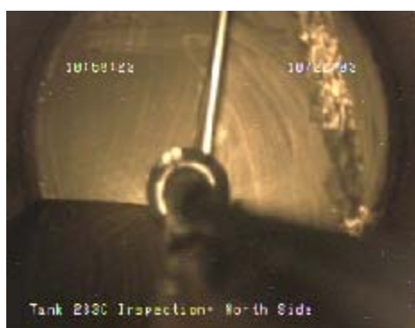
Figure 8: Sludge and Salt Build-up on Internal Tank Walls
