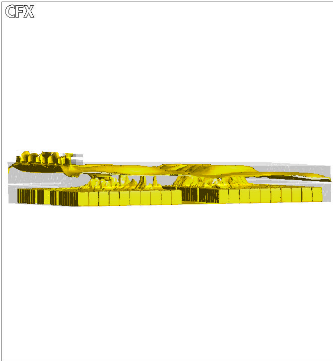
Figure 4: Isosurface of 35 °C temperature showing shape of hot layer strata (temperatures greater than 35 °C lie above and inside yellow surfaces)
