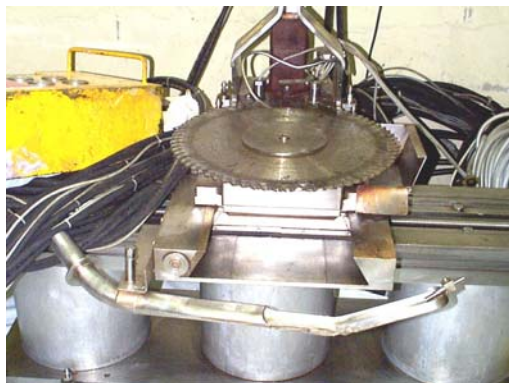
Pictures 1 and 2: The two main mechanical cutting techniques used for the dismantling of the reactor internals and the reactor pressure vessel
