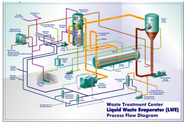
The distillate water from the evaporators is sent to holding tanks where it is acceptance tested for release. If the distillate passes testing, the water is discharged to the process sewer, which discharges to the Ottawa River. The immobilized bitumen waste is transported to a waste management area for dry-storage management.
